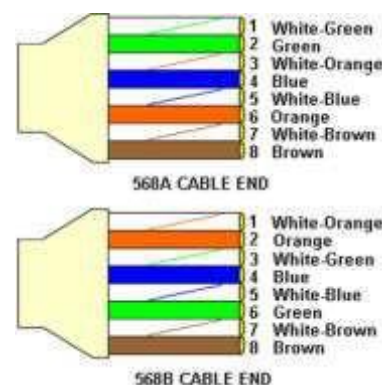
Figure 3.9: EIA/TIA 568A and 568B
